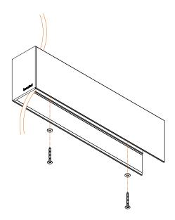
Slide in alignment brackets halfway into the profile and tighten them using an allen key and provided headless screws.
