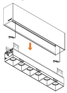
Insert the main electrical cable into the profile.
