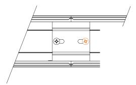
► Fix the second fixture to the surface using the specified screws and washers.
